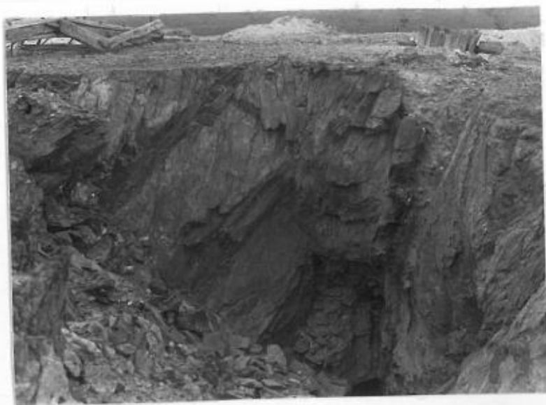
Fig.22 Looking south into the open pit, Aclare Mine. Two pelitic layers on the left (east) trend up into the ore, which has a schistose wall on either side. The ore has internal isoclinal folds, (not quite visible). It apparently lies on the western limb of an anticline, which is parallel to the schistosity. A southerly plunging syncline is clearly visible on the right. For scale depth is about 95 feet.
