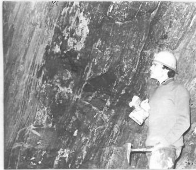
Fig.21. Ore - wallrock contact, Aclare Mine, looking south in adit at main shaft. Ore is the stained, layered material to the right, wallrock is unstained mica schist.
