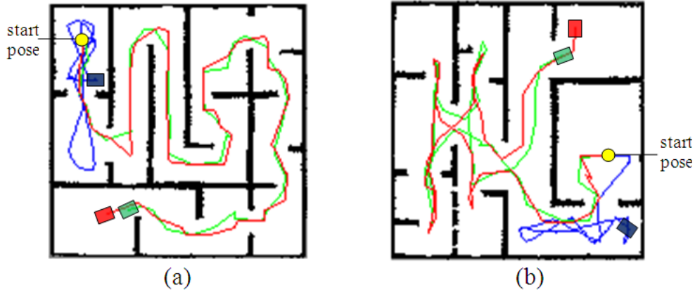
Figure 6.16: Application maps showing footprints of the robot using three different scoring function: red line for STRUC_EVO, green line for FUNC_EVO, and blue line for CONST_EVO (a) Robot pose on environment 1 after 240 seconds run-time (b) Robot pose on environment 2 after 234 seconds run-time.
