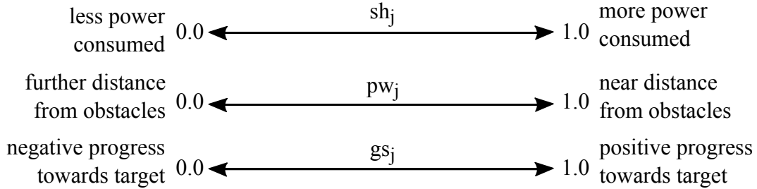
Figure 6.17: A description of state signals. A sampled state signal has a value between 0.0 to 1.0.
