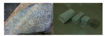
Figure 4.26 Block of Kanmantoo Blue stone and preparation of cubic specimens [after Dong et al., (2011)]
