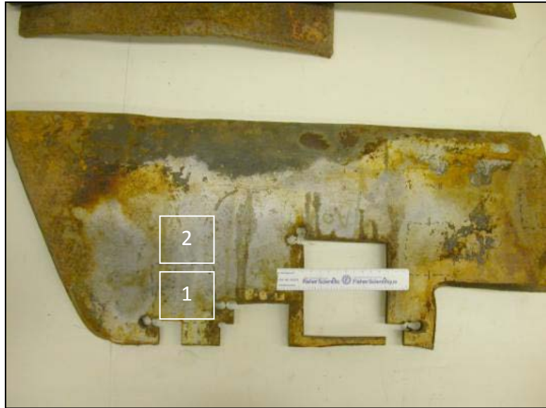
Figure 2-10: Locations of the crack colonies on the pipe panel for the TransCanada study (Xie et al. 2009).
