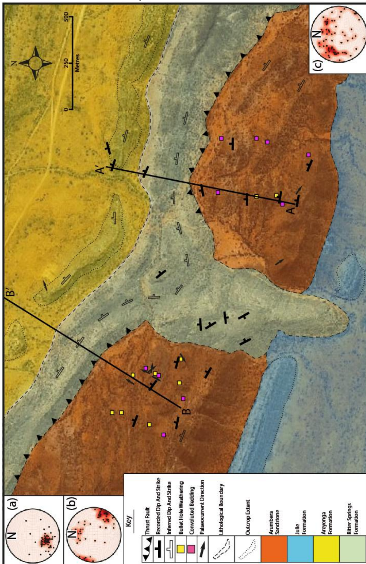
Figure 2: Geological map of the studied salt diapir in the Amadeus Basin, central Australia. The location is approximately 90 kilometres east of Alice Springs. The map includes the lithological units encountered as well as the location of convoluted bedding, bullet hole weathering and palaeocurrent directions calculated from sedimentary structures. Stereonets include (a) poles to bedding for the Arumbera Sandstone, (b) poles to fracture planes for the Arumbera Sandstone on the western flank of the diapir and (c) poles to fracture planes for the Arumbera Sandstone on the eastern flank of the diapir. Cross sections A to A' and B to B' are included in Figure 13.
