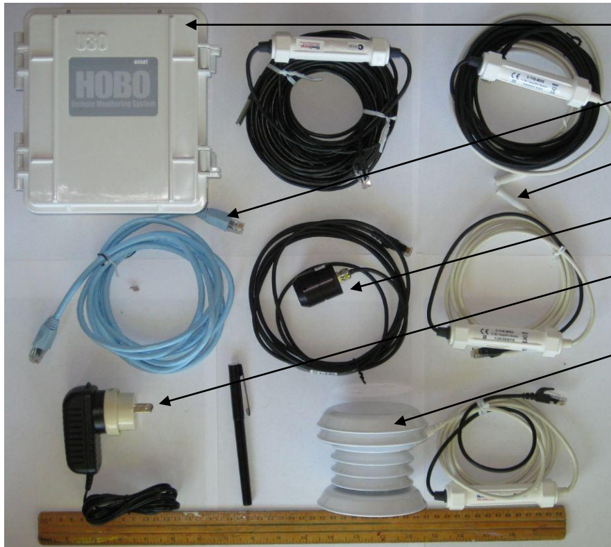
Figure 2 - Remote monitoring system which hooks up to internet
