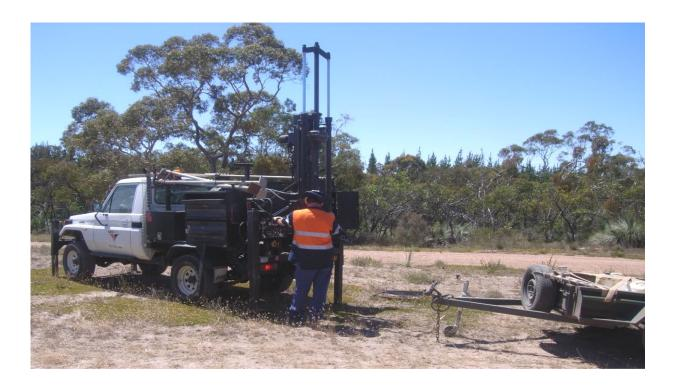
The push core drilling rig used to measure regolith depth in the Adelaide Hills, South Australia. A combination of existing site data, new drilling and field measurements (e.g. road cuttings and gullies) were used to develop a predictive model of weathering depth in the region.
