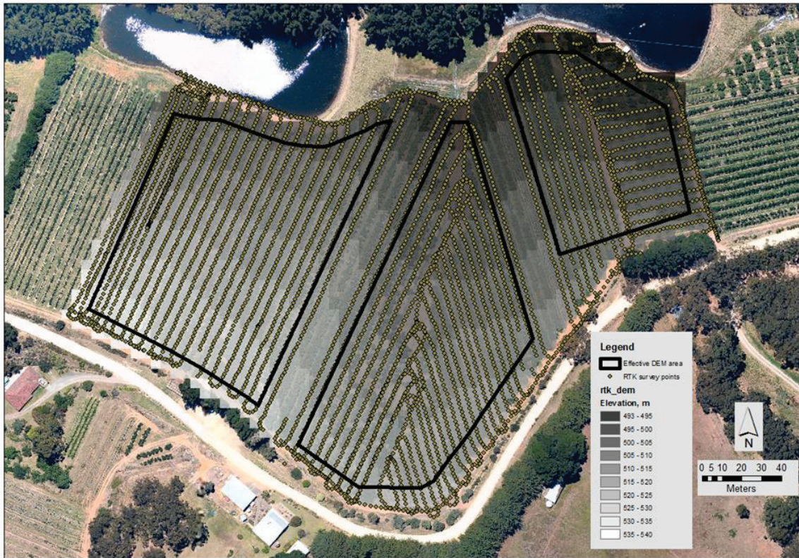
Figure III.e. Survey points and digital elevation model from real-time kinematic global positioning system (RTK-GPS) survey.
