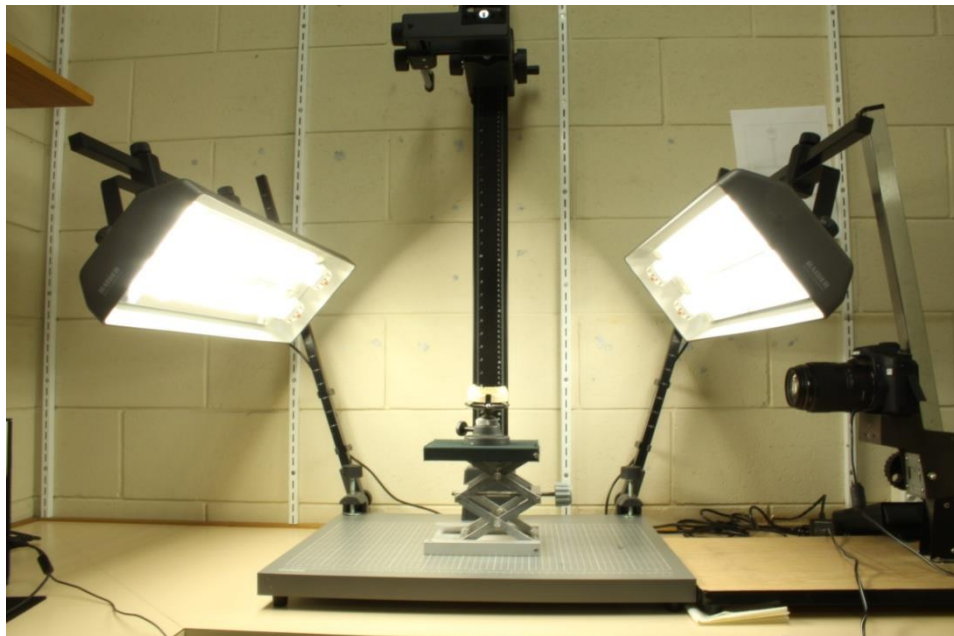
Figure 4.2. 2D imaging system used to assess infraocclusion.
