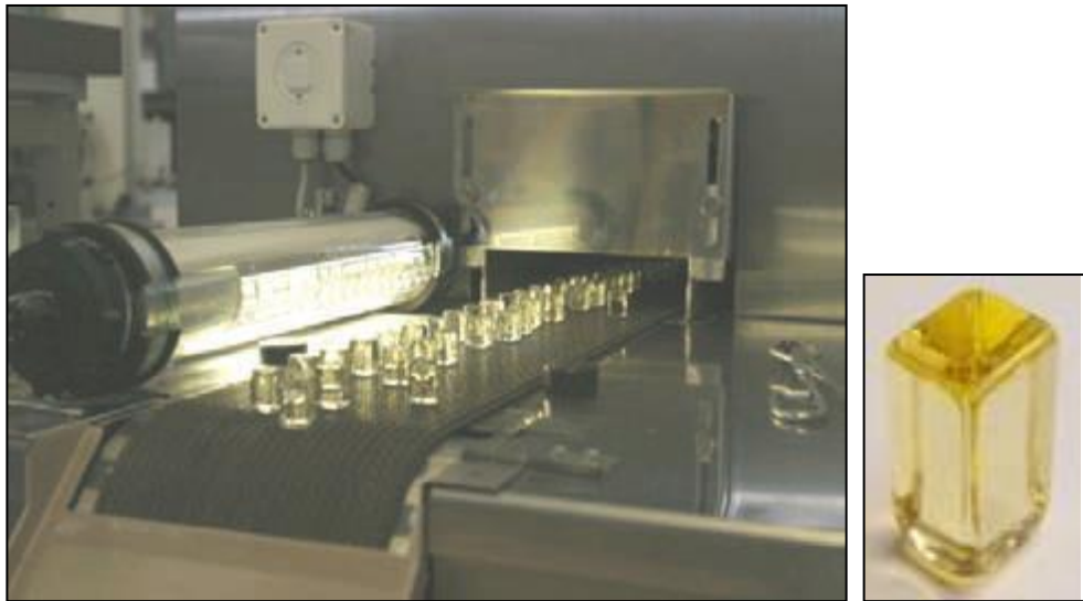
Figure 5.9: The translucency of IPS e.max. (Ivoclar Vivadent, Schaan, Liechtenstein) aids ease of quality control since porosities can be easily detectedSource: R&D Ivoclar Vivadent AG, Schaan, Liechtenstein.
