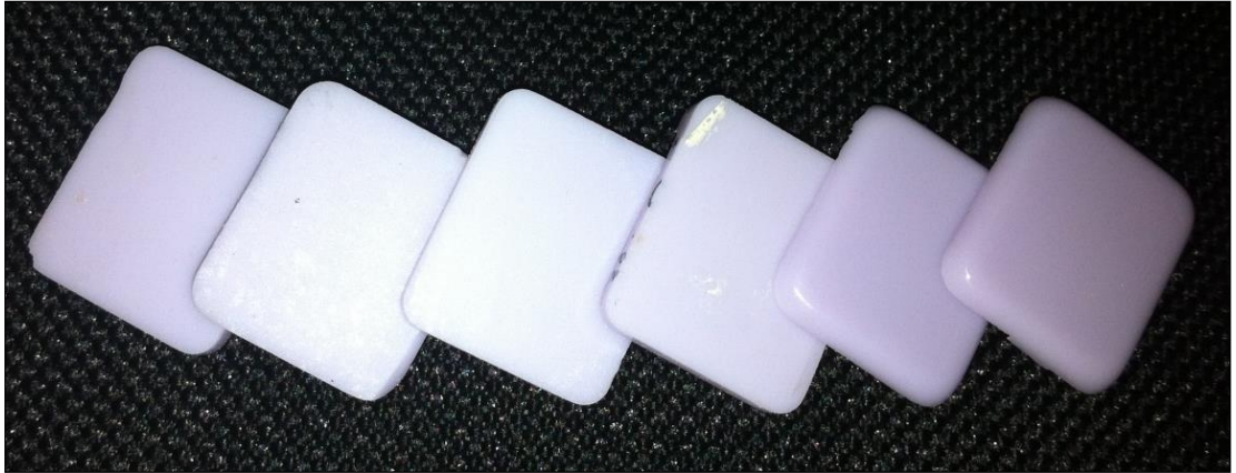
Figure 9.1.6: Sectioned IPS e.max CAD block into 2mm thick slices.
