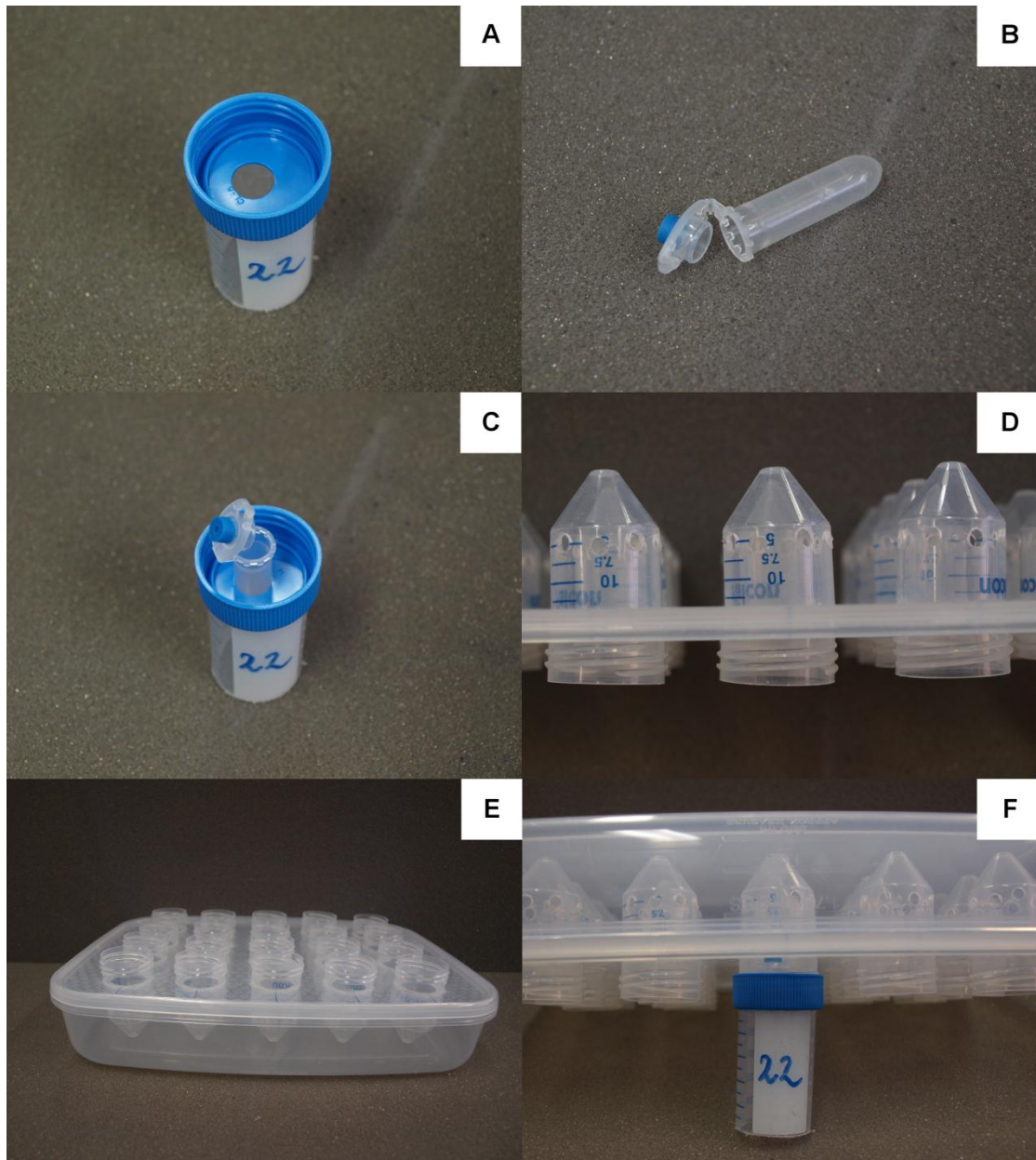
Figure 10. Close-up views of the custom-made transpiration chamber: (A) Socket for the Eppendorf tubes; (B) Eppendorf tube with rubber seal; (C) Assembled berry holder unit; (D) Lid of the transpiration chamber with individual berry cells; (E) Complete transpiration chamber (upside down); (F) Transpiration chamber with one berry holder unit attached.
