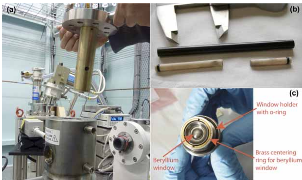
Figure 2.2 Pictures of mAESTRO autoclave: (a) the autoclave body and heating block; (b) internal glassy carbon cell with two alumina pistons; (c) Beryllium window and holder.
