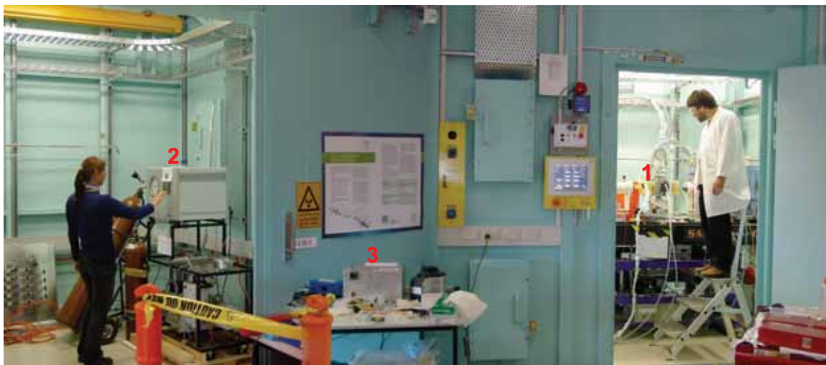
Figure 2.5 mAESTRO system at the XAS beamline of Australian Synchrotron (1: mAESTRO autoclave in the first experimental hutch, 2: pressure generation-regulation unit in the second experimental hutch, and 3: temperature control unit near the control cabin).
