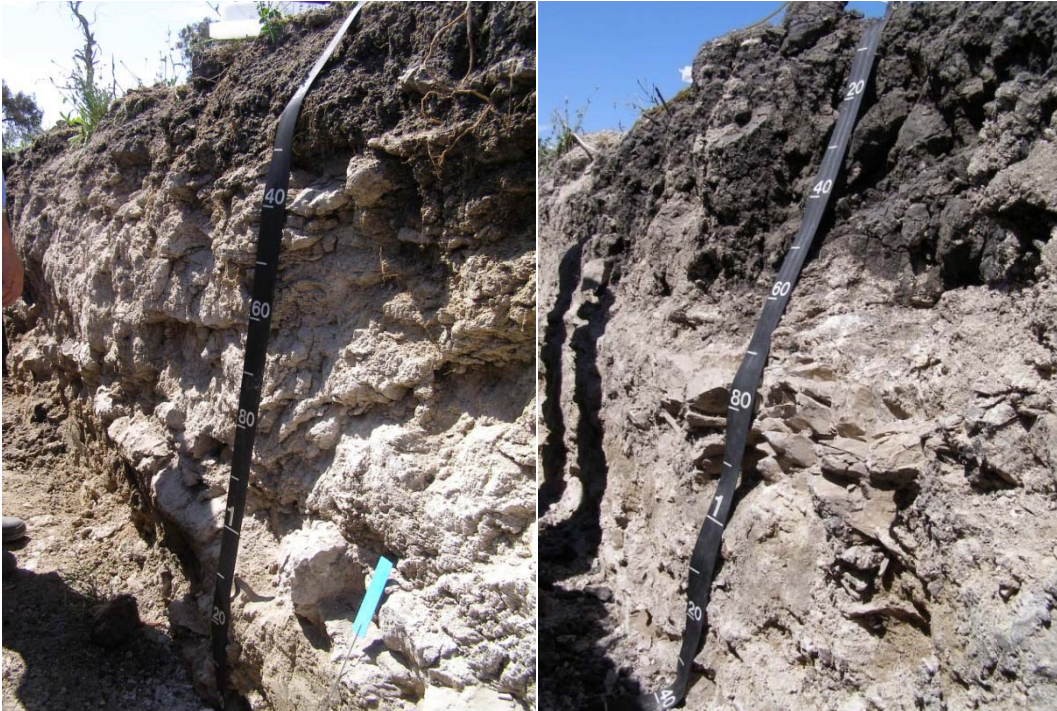
Fig. 6.1 Photographs taken within the trench showing the major soil type, Chromosol, (left) and the deep black Vertosol that occurred in isolated areas within the trench (right).
