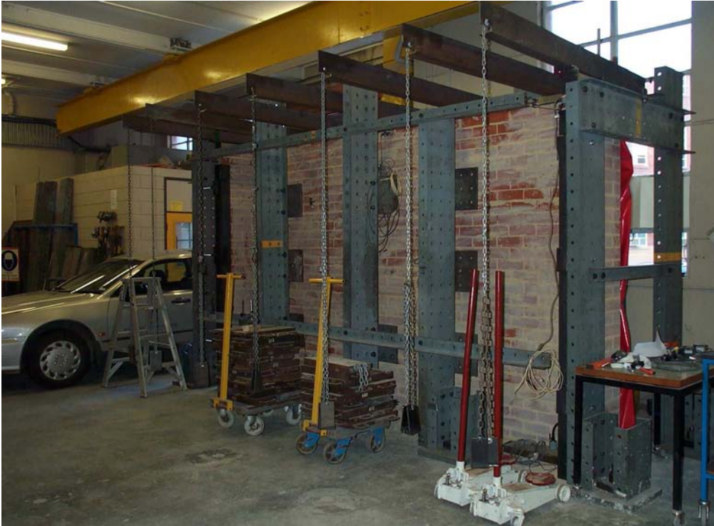
Figure 2.9: Photograph of the overall test setup, including precompression arrangement (wall s1 shown).
