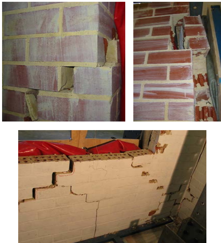
Figure 2.28: Examples of sliding between adjacent sub-plates within the mechanism.
