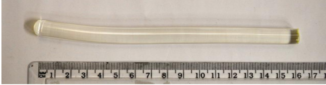
Figure 32: Undoped TZNL glass rod generated from the extrusion of a 100g glass billet.
