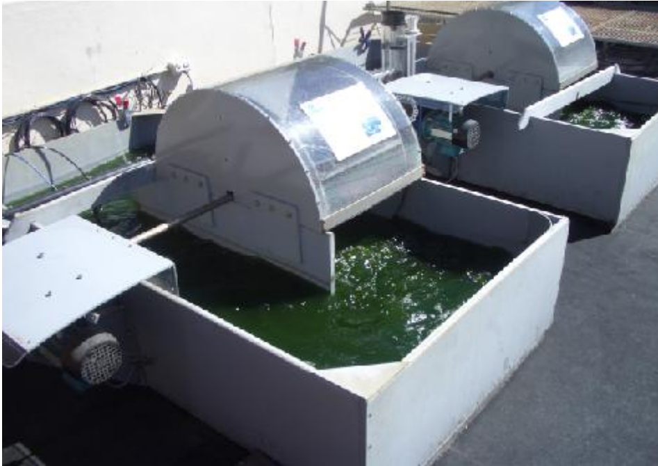
Figure 3.4 Cultures of MUR230 and MUR232 inoculated in the outdoor raceway ponds upto 400L from 15L inoculum
