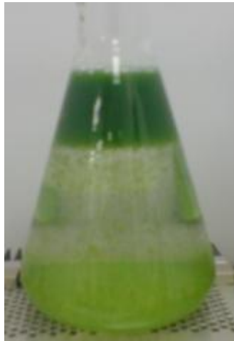
Figure 4.9 Electroflocculation with Aluminium electrodes
