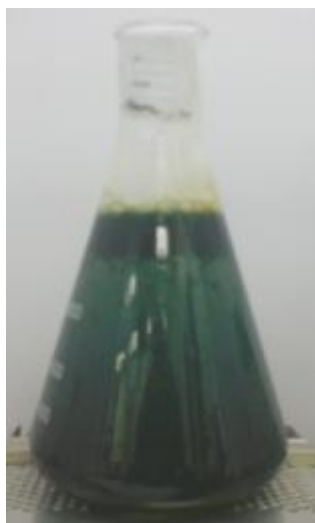
Figure 4.12 Electroflocculation with Bronze electrodes
