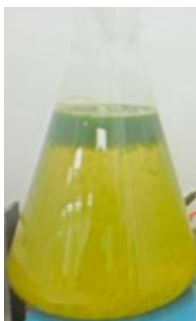
Figure 4.6 Electroflocculation with SS-304 electrodes
