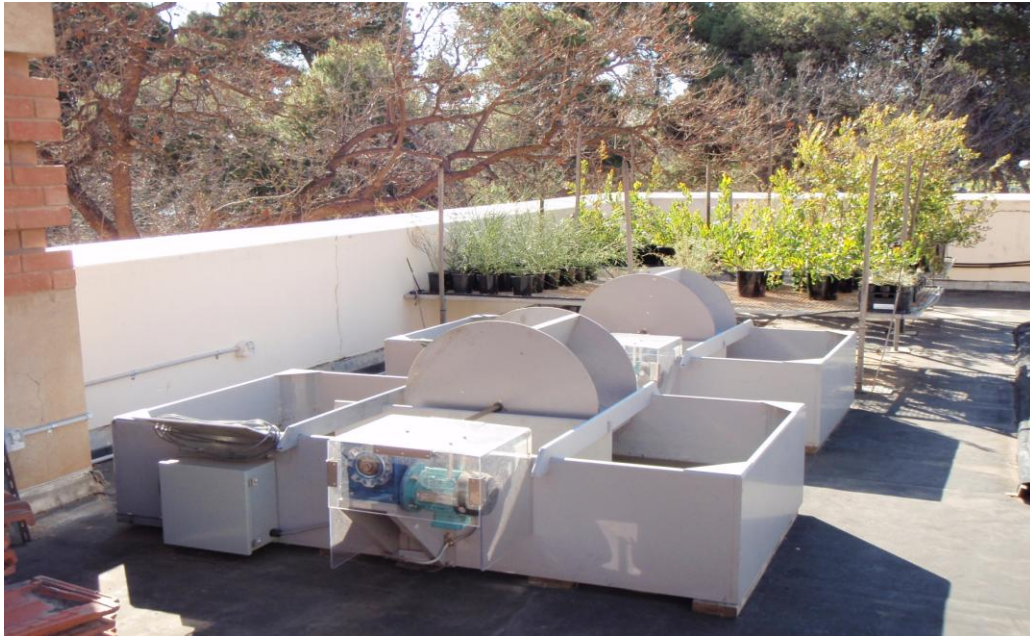
Figure 3.3 Outdoor raceway ponds located on the roof, at University of Adelaide
