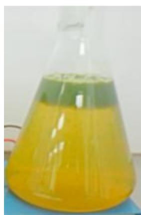
Figure 4.7 Electroflocculation with SS-316 electrodes
