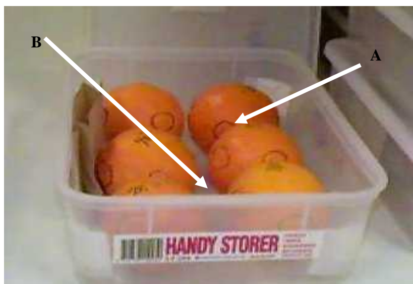
Figure 6.2 Fibre position for analysis of headspace concentration of citral in the box at each temperature when (A) positioned above the fruit and (B) positioned below the fruit
