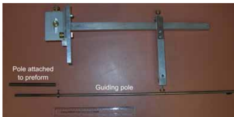
FIGURE 4.9: Guiding pole used to force the leading edge of the wedged-jacket extrusions along a straight line.
