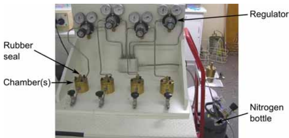
FIGURE 5.25: Pressure filling setup used to coat the internal surfaces of MOFs. The fibre is inserted into the rubber seal using a syringe. A sample vial is then positioned into the chamber, which is closed before applying pressure via the nitrogen gas bottle and regulator.
