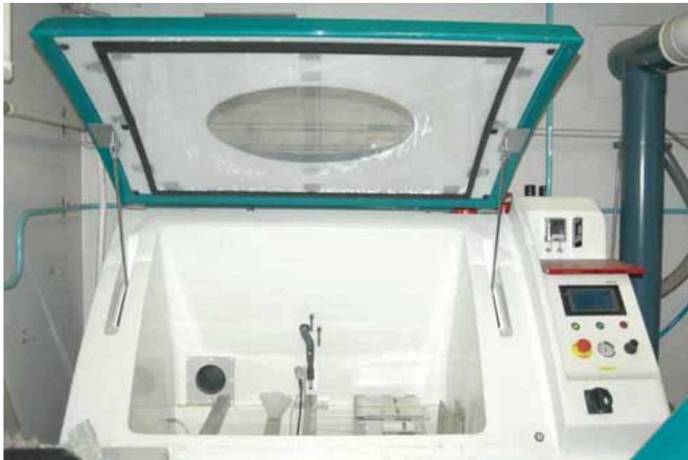
FIGURE 5.14: Salt spray chamber used to accelerate the rate of corrosion of the aluminium lap joints.
