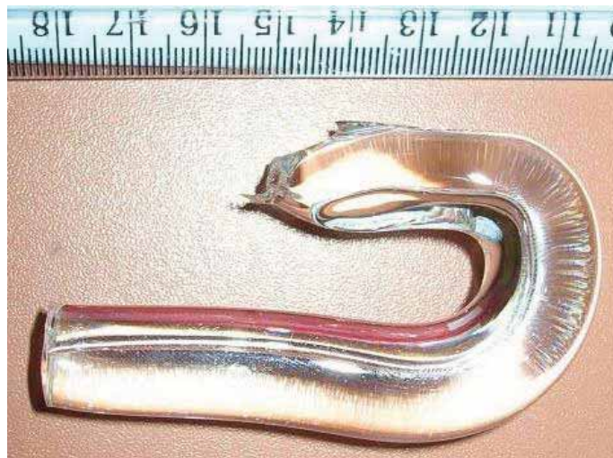
FIGURE 4.8: Bent wedged-jacket preform with a 45^\circ wedge where the left hand side was the last to exit the die.
