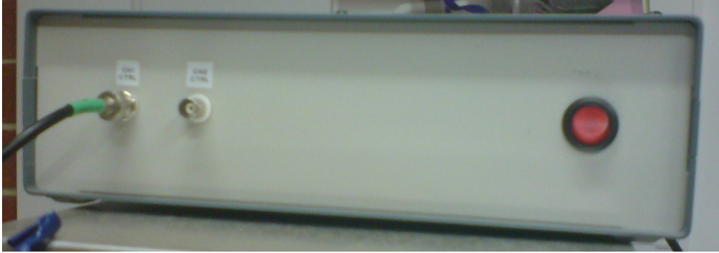
Figure 11. The power controller of dryer lamps
