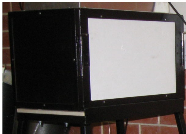
Figure 5. The walls of the dryer made by Insulation boards and steel sheets
