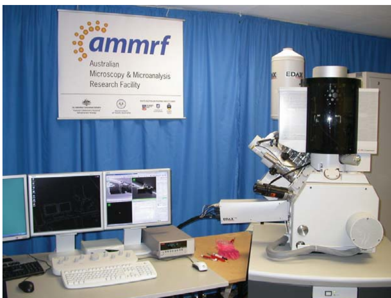
Figure 5.9. Images of FIB milling machine. Image of focused ion beam milling machine, Helios NanoLab 600 from FEI, used for cleaving porous fibres.
