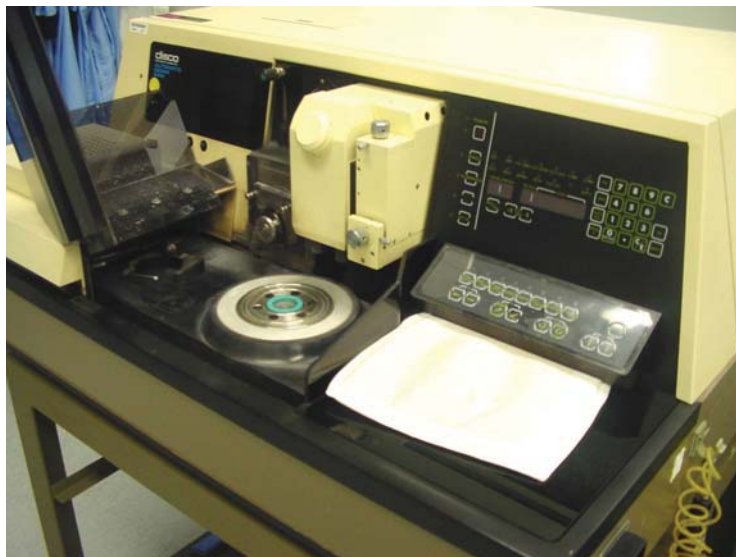
Figure 5.7. Images of SD saw machine. The image of semiconductor dicing saw machine, DAD-2H/6 from DISCO, used for cleaving porous fibres.
