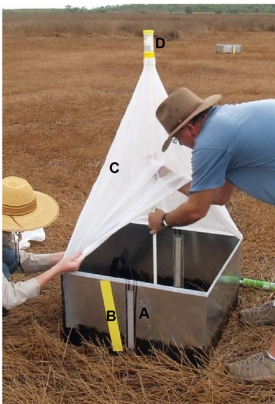
Figure 2 Emergence trap design: mesh-covered holes allow tidal flooding without larval movement (A); yellow magnets applied over holes prevent unwanted larvicide entering trap (B); mesh emergence tent prevents unwanted species’ oviposition inside trap (C) and also catches emerging adults (D).
