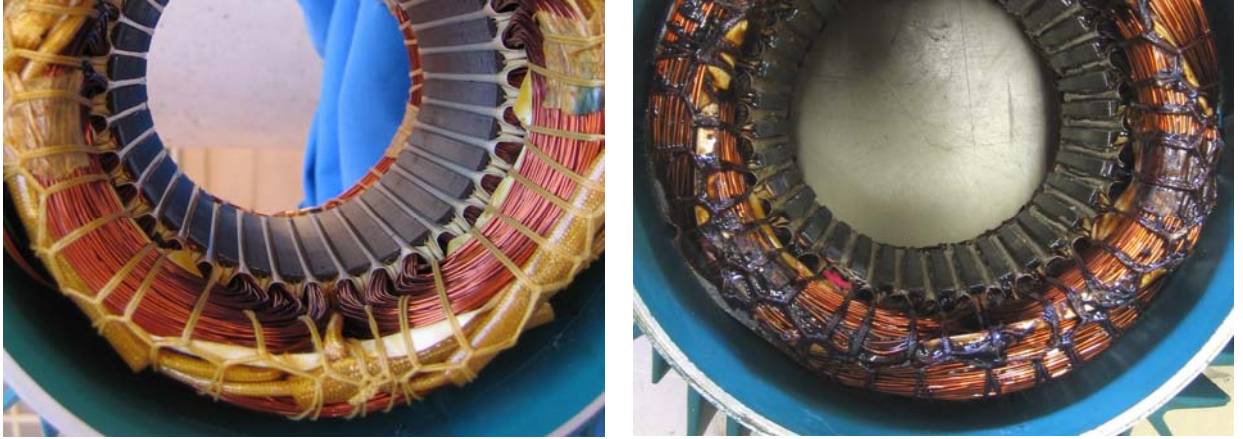
Figure 6-2 The inside of the stator a) before compression of the stator winding and b) after compression and machining.
