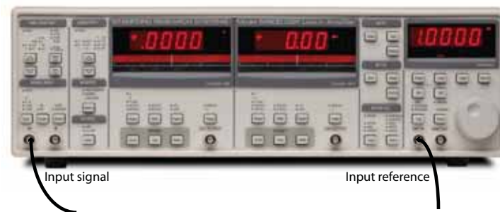
Figure C.4. Photograph of SR830 lock-in amplifier. This figure shows the photograph of the SR830 model lock-in amplifier.
