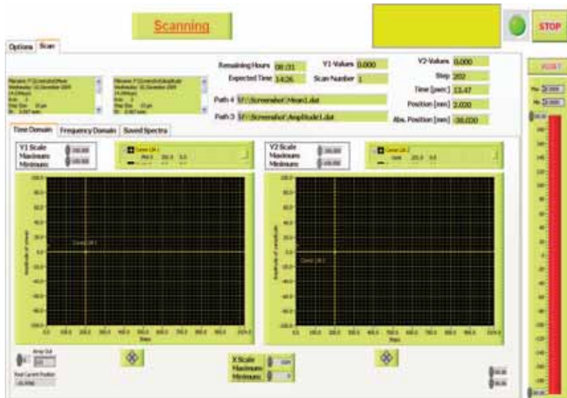
Figure C.10. Screen shot of LabVIEW program for double-modulated THz-DTDS spectrometer. This is a screen shot of the LabVIEW program developed to control the double-modulated THz-DTDS spectrometer. With this program, one may acquire mean and amplitude data simultaneously for analysis purposes. The graph indicators for acquiring the mean and amplitude signals are shown in the figure.
