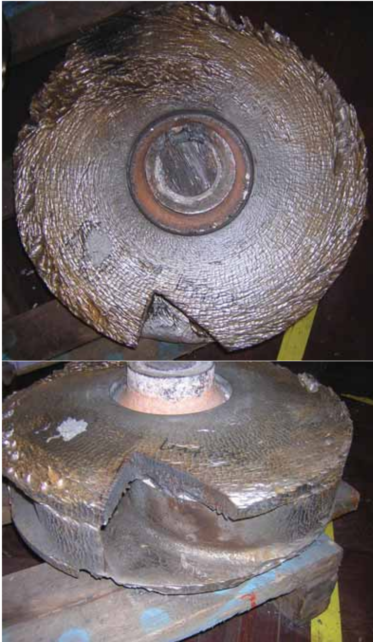
Figure 4.1: (a) Overview of the ex-service alumina plant slurry pump impeller designated as HypoA. The wedge removed from the casting indicates the sample location. (b) The wear surface of the HypoA impeller casting showing the scalloped wear surface appearance over the entire wear surface.
