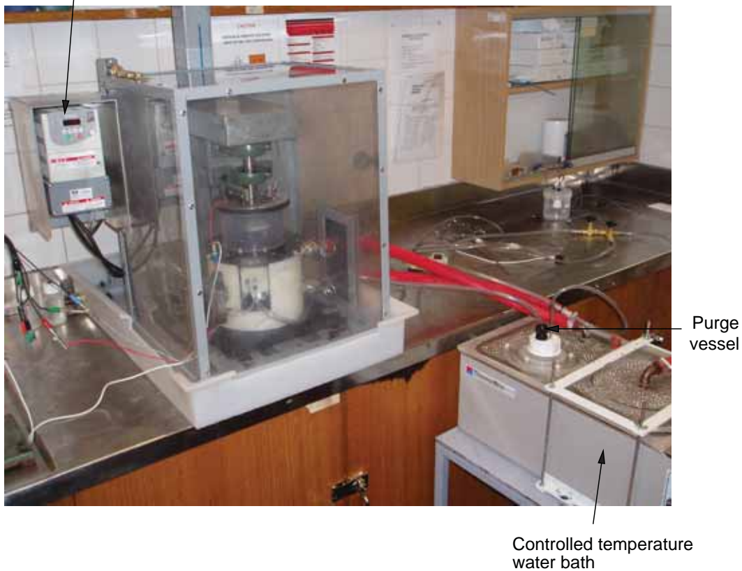
Figure 2.10: General overview of the assembled electrochemical erosion-corrosion test apparatus showing enclosed test section, rotational speed controller and water bath.
