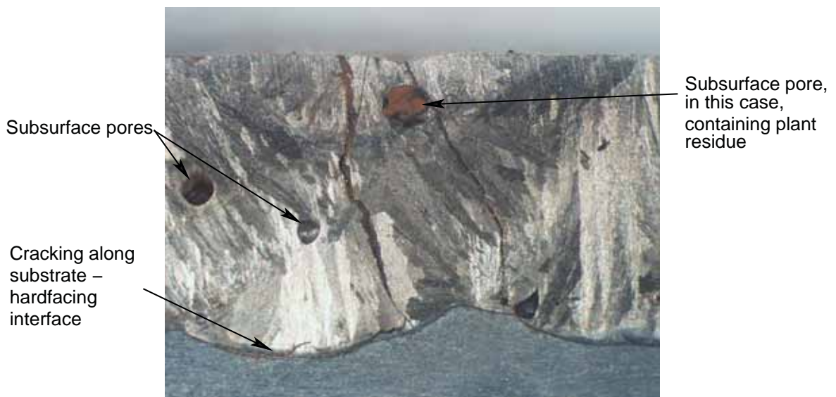
Figure 4.12: Check cracks in a transverse sample that extend to the substrate-hardfacing interface and continues to extend along the substrate-hardfacing interface. Subsurface pores were often found to contain plant residue because they had been intersected by a check crack. The appearance of the overlay is due to the sample being lightly etched acid ferric chloride.
