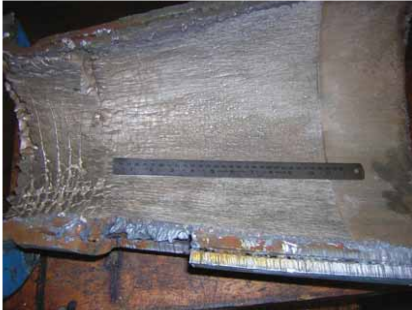
Figure 4.6: Overview of the ex-service alumina plant trumpet spool designated as WeldoverlayB.
