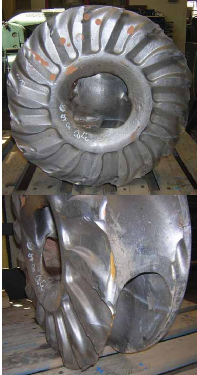
Figure 4.2: (a) Overview of ex-service alumina plant slurry pump impeller designated as HyperA. (b) The wear surface of the HyperA impeller casting showing the accelerated wear at the periphery of the impeller.
