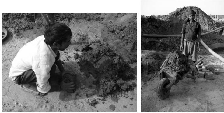
Fig. 7.39a. Tempering and mixing of clay done by hand before being transported for moulding. (Source: Photograph by author, Ahmedabad, 2007.)
