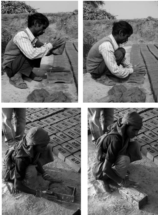
Fig. 7.39b. Moulding process includes throwing the clay mix into metal mould, and shaping by hand. (Source: Photograph by author, Ahmedabad, 2007.)
