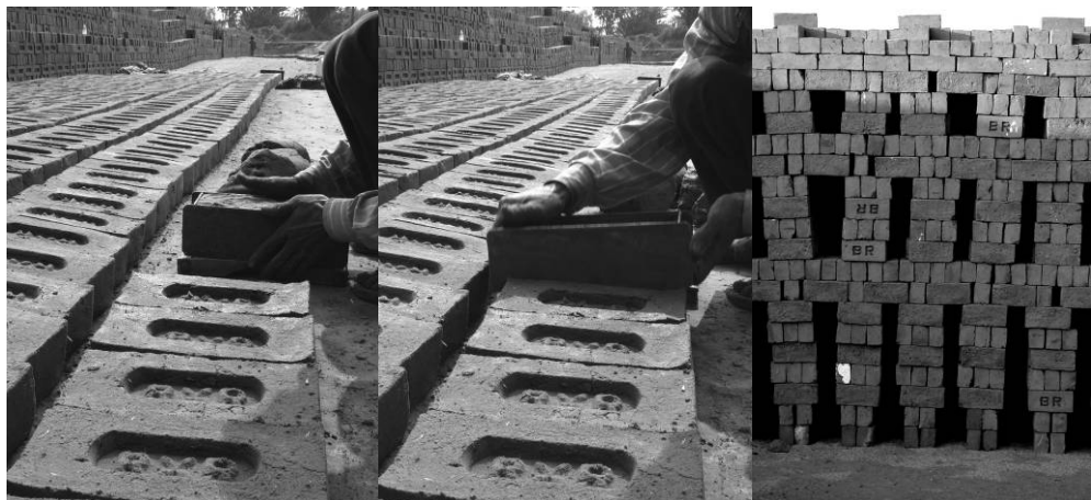
Fig. 7.39c. Brick is turned out of the mould and stacked for drying before firing. (Source: Photograph by author, Ahmedabad, 2007.)
