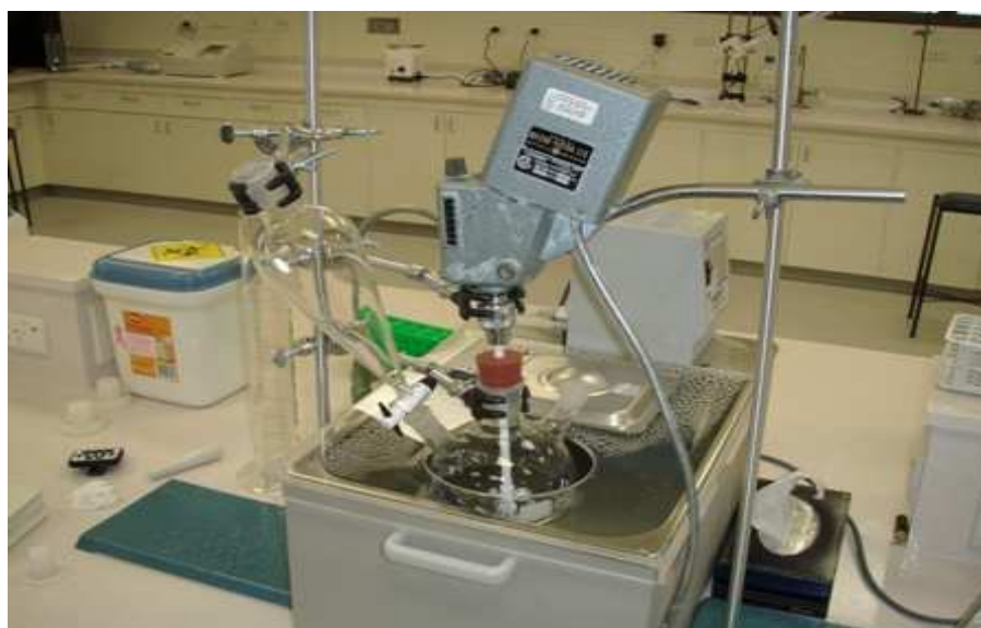
Figure 1: Experimental setup for the synthesis of TiO 2 -K catalyst particles.
