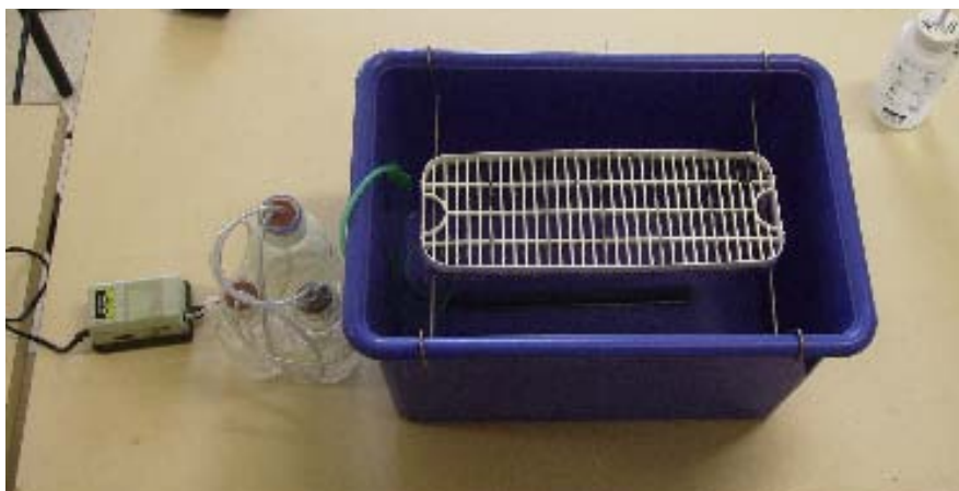
Figure 3:15: Hydroponic screening equipment, including aqua pump, KOH solution bottles, 25L tank, stainless steel rods, airstone and plastic seed tray with mesh.
