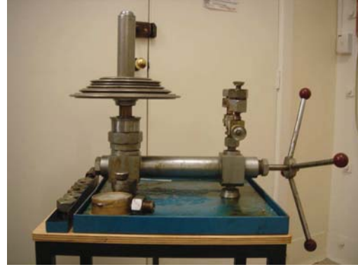
(b) Dead-weight Pressure Tester
