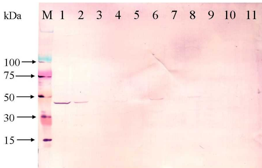
Figure 2-10 Comparison of expression levels in M9 media at different growth temperatures and induction times. M, Colour marker, 5 \mu L (Sigma) and 6xHis ladder, 2.5 \mu L (Qiagen); 1, WCE, 30°C, 3 h expression; 2, WCE, 22°C, 3 h expression; 3, soluble fraction, 22°C, 3 h expression; 4, WCE, 22°C, 20 h expression; 5, soluble fraction, 22°C, 20 h expression; 6, WCE, 4°C, 3 h expression; 7, soluble fraction, 4°C, 3 h expression; 8, WCE, 4°C, 20 h expression; 9, soluble fraction, 4°C, 20 h expression; 10, WCE, 4°C, 26 h expression; 11, soluble fraction, 4°C, 26 h expression. Lanes 2-11 - equivalent of 300 \mu L culture, all grown to OD 600 of ~0.6 then induced with 0.1 mM IPTG.
