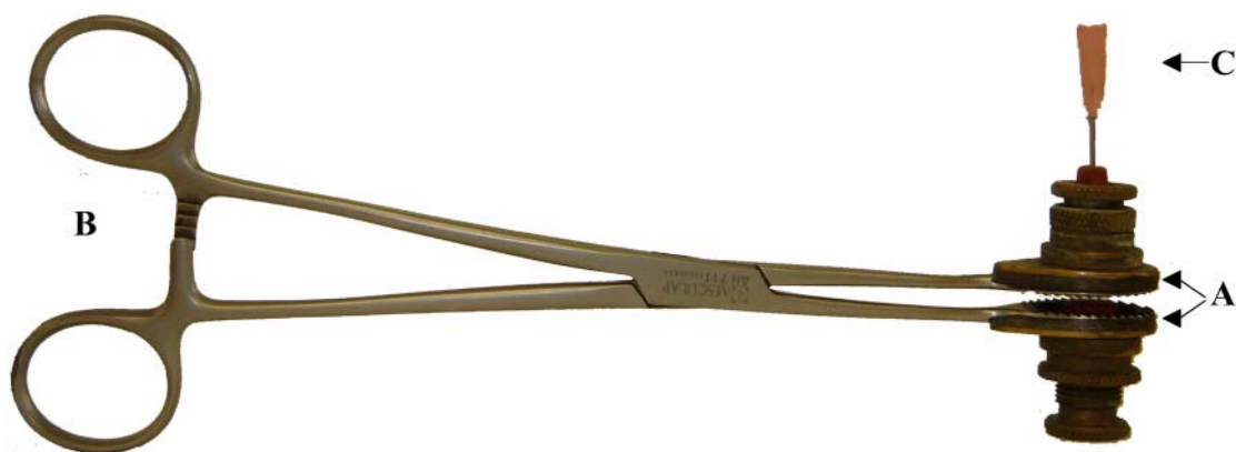
Figure 2.1 The Hagborg device used for bioassay of attached barley leaves. The leaves were put gently between the rubber stoppers (A) and kept still by locking the forceps (B). The samples were injected using a 1 mL plastic syringe attached to part C.
