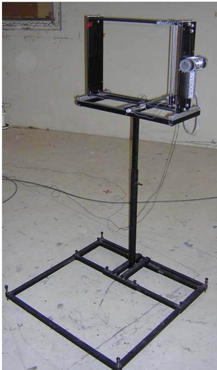
Figure 3.4: Automated traverse used to position the microphone during experiments.
