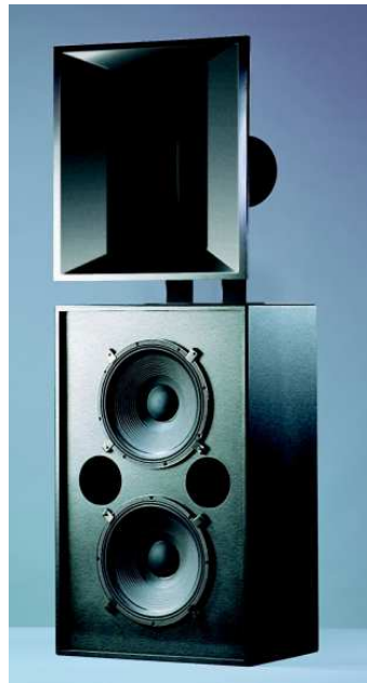
Figure 2.2: Commercially available cinema loudspeaker system. The horn loaded loudspeaker is mounted on top of a low frequency direct radiator loudspeaker, and the system is located behind the cinema screen.
