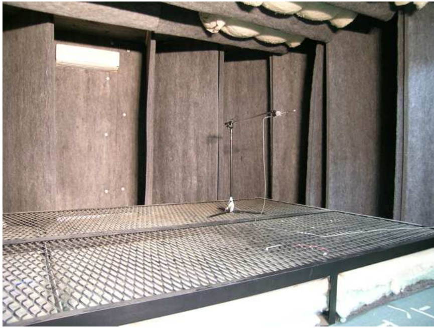
Figure 3.2: Semi-anechoic facility showing wedges of acoustic absorptive material.
