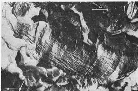
Fig. 2. Electron micrograph of the fracture surface of Willaloopa illite core obtained using a replica technique. Arrows indicate the direction of uranium shadowing
