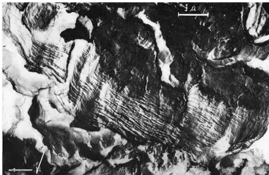
PLATE 1.—A electron micrograph of a replica of the fracture surface of a clay core of Willalooka illite. The arrows show the direction of shadowing. The interleaved and parallel arrangement of the clay crystals can be seen to extend over a considerable distance indicating that a domain is considerably more complex than the simple model.
