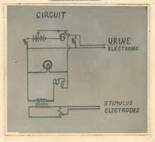
Eight to Ten volts (8-10) from a dry battery (No. 761) are sufficient for the relay circuit. Four and a half to six volts (48-6) are ample for the secondary circuits. Patients vary in both their skin resistance and their sensitivity to the applied stimulus so that potentiometer needs to be able to vary the stimulus up to about 70 volts in actual use.
