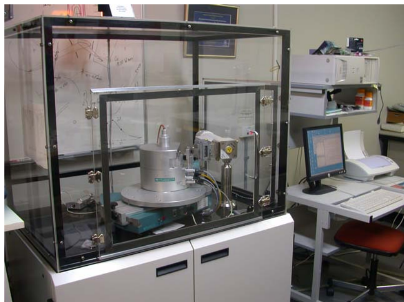
Figure 3.4. Huber HTC 9634 X-ray diffractometer used in this work, with Co K_{\alpha 1} radiation ( \lambda = 1.78897 \text{ \AA} ).
