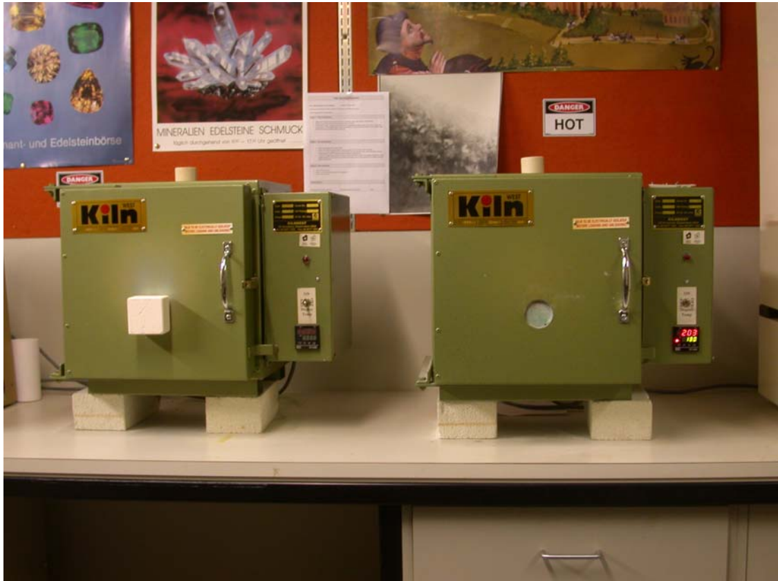
Figure 3.1. The muffle furnaces used in this work, BC9090 (Kiln, Co. Ltd.). The safe operating temperature range is below 1200°C. The heating schedule is programmable.
