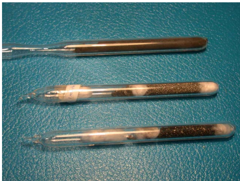
Figure 3.3. Sealed glass tubes (bottom two) filled in with charges and covered with silica wool at both ends. Open tube filled in with finely ground powder charge (top).
