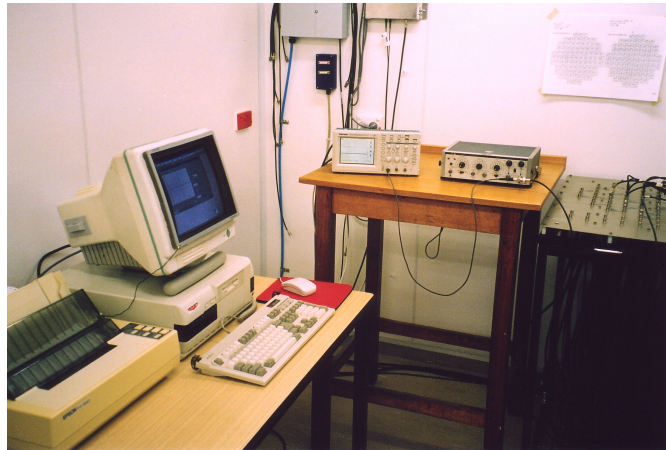
Figure 3.1: Photograph of TDR equipment system I. The system test equipment comprises printer (from left), IBM compatible PC, TDS 210 digital storage oscilloscope and AE PG58 pulse generator. This is connected to the device under test via the Cable-Balun-Antenna patchboard (far right).
