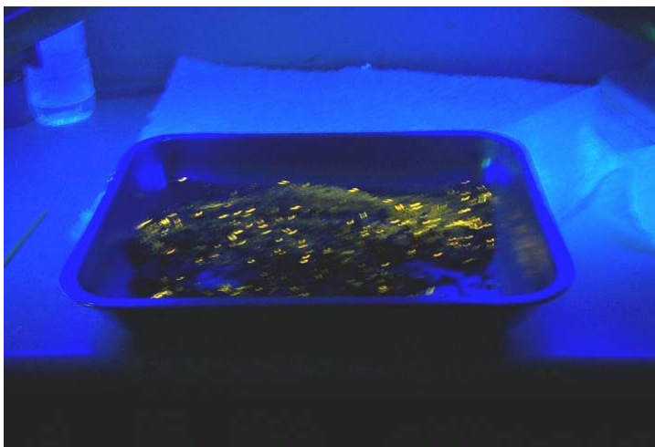
Figure 5.3. Fluoresced seeds of annual ryegrass under ultraviolet light in a dark laboratory room.
