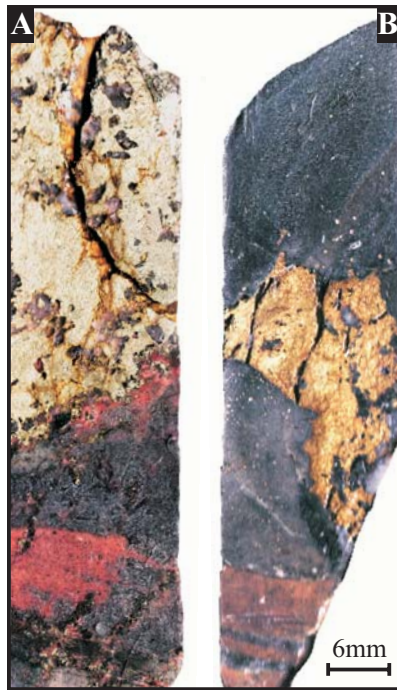
Figure A8.13. Representative samples from Polygonum prospect. Sample taken from diamond drillhole SR1. Sample numbers in italic . (a) SR1A - 338m; (b) SR1C - 504.8m. Scale same for each sample block.
