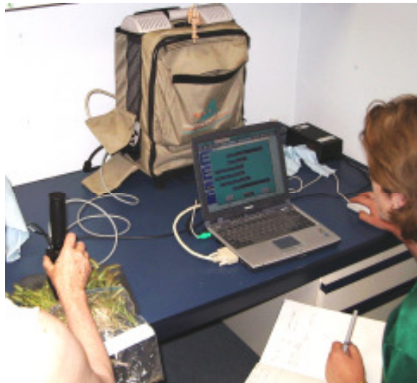
Figure 3-3 Method for collecting spectra from soil and plant samples in the laboratory
