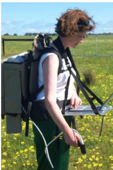
Figure 3-1 Collecting spectra in the field with the portable spectrometer
