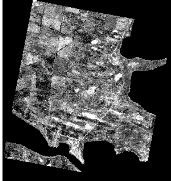
Figure 5-7 MTMF result using mean saltpan reference spectrum. Bright salt pans are dispersed throughout the central and coastal discharge areas. The main Site A pan is not clearly mapped.
