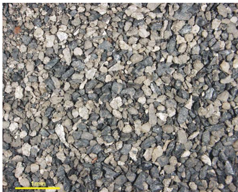
Figure 6.8 Cuttings from a Unit V black carbonaceous siltstone in Trumpet-1 (1268-1280m). Calcite is present as white to light gray fragments.
