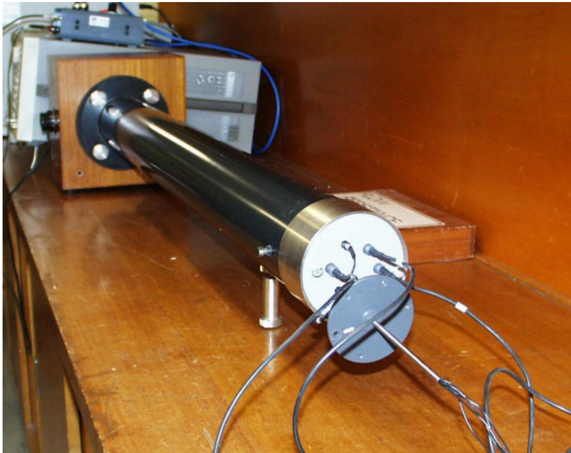
Figure 3.10: Photograph of the experimental set-up to select phase and sensitivity matched microphones
