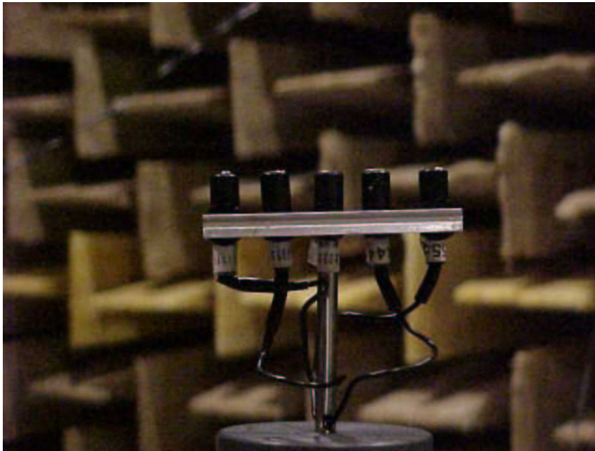
Figure 5.4: Photograph of the extended microphone array (with five elements) used in higher-order virtual microphone real-time experiments
