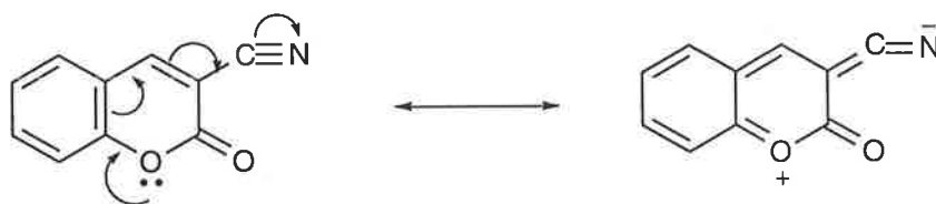
Figure 3.2: General resonance structures of coumarin nitriles indicating the delocalisation of electrons which decrease the susceptibility for nucleophilic attack by L-cysteine.
