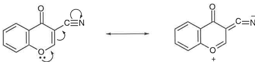
Figure 3.1: Resonance structures of nitrile 25 indicating the delocalisation of electrons which decrease the susceptibility for nucleophilic attack by L-cysteine.
