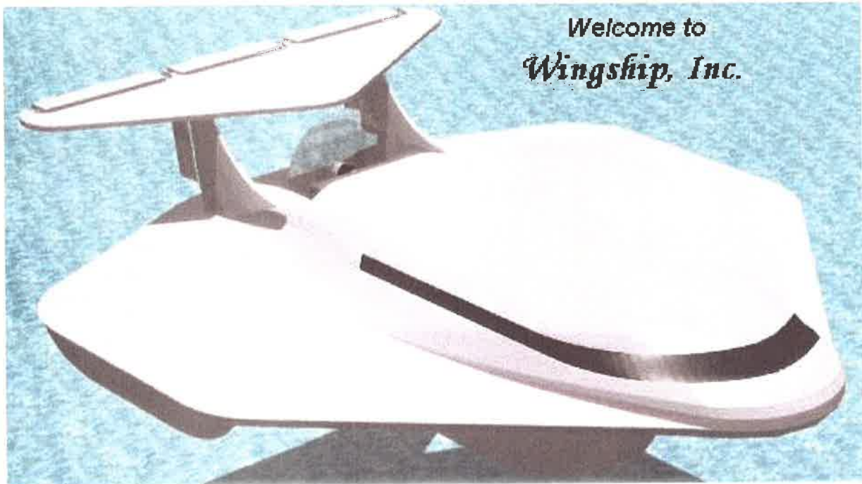
Figure 4.4: The proposed Wingship Hoverplane concept ground effect vehicle. The Hoverplane is expected to be large enough to be able to fly safely above 8 metre waves. Reproduced with permission.
