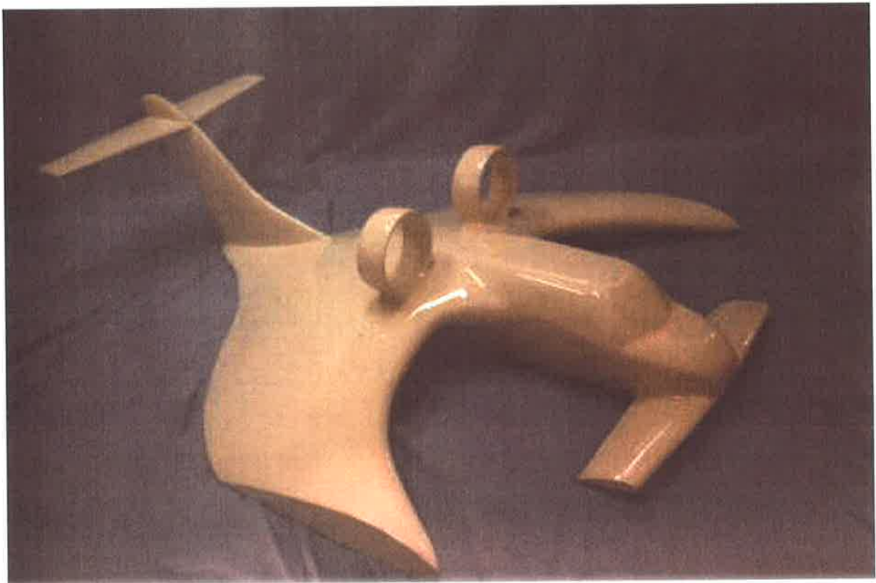
Figure 4.3: The RADACorp C-850 shows the trend in future designs for ground effect vehicles. Although integrated wing-body designs are more complicated for aerodynamic analysis, they offer superior parasite drag characteristics and market appeal. Reproduced with permission.
