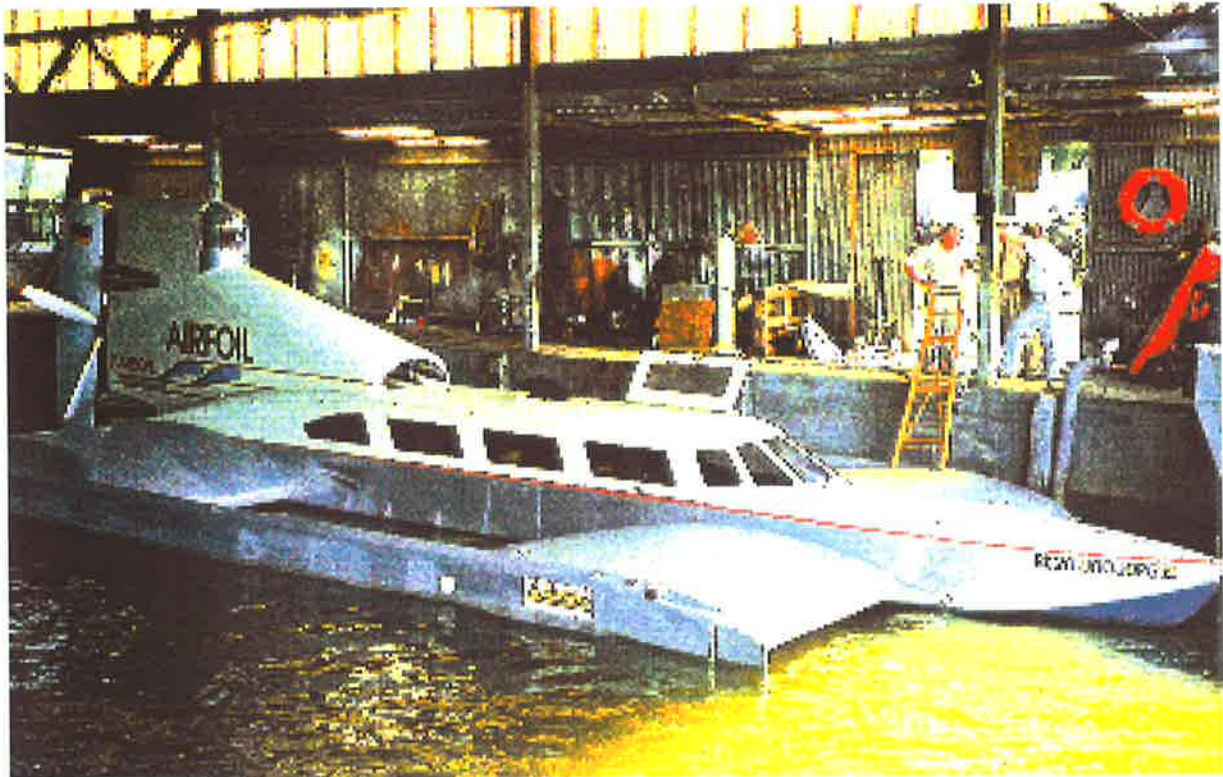
Figure 4.14: The tandem-wing design of the Jörg TAF VIII is used to counteract the natural pitch-heave instability of a single wing in ground effect.
