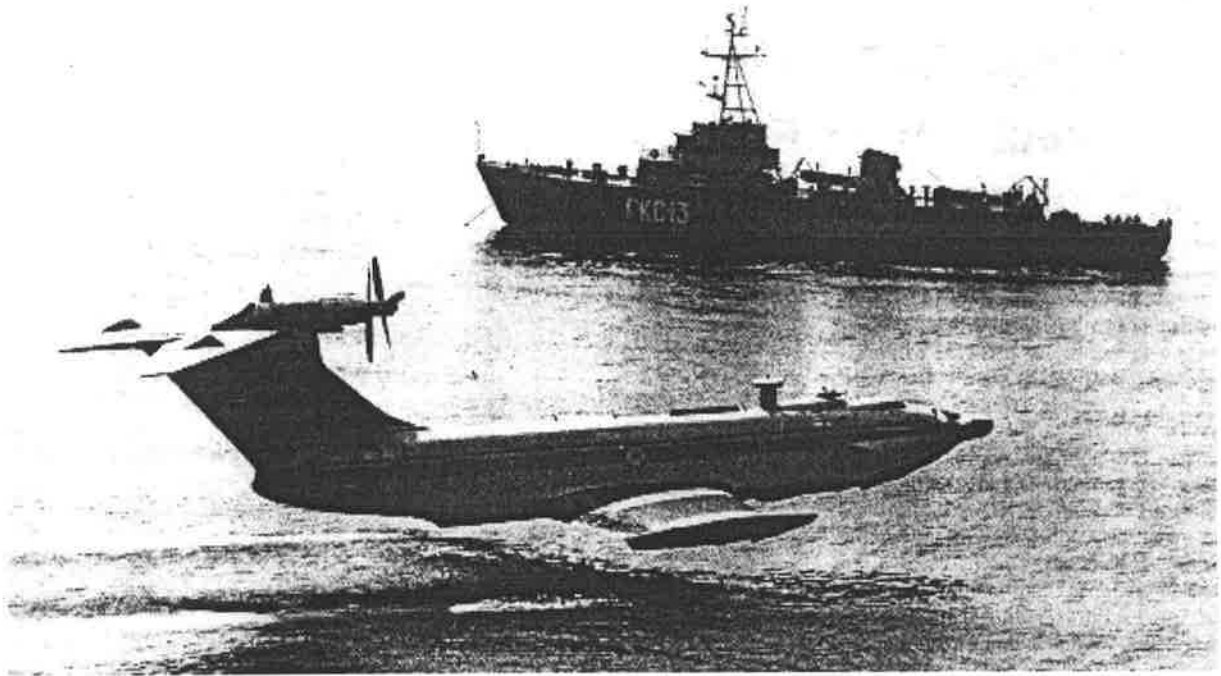
Figure 4.2: The 120 tonne “Orlyonok” is one of the largest Russian ekranoplans. First launched in 1972, it has a length of 60 metres, a cruising speed of 400 kilometres per hour and a range of 1000 kilometres. Reproduced from “Engineers Australia” (1996).
