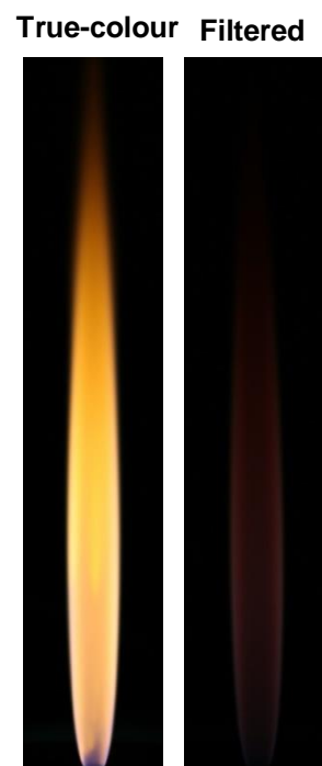
Figure 4: Photographs captured with and without the notch filter for undoped jet flame (JET-T0).
