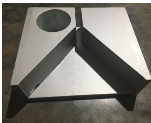
FIGURE 25 Flume to be installed in 2020 at one of the flow monitoring weirs at Dalhousie Springs (Photo: F Mangeruca)
