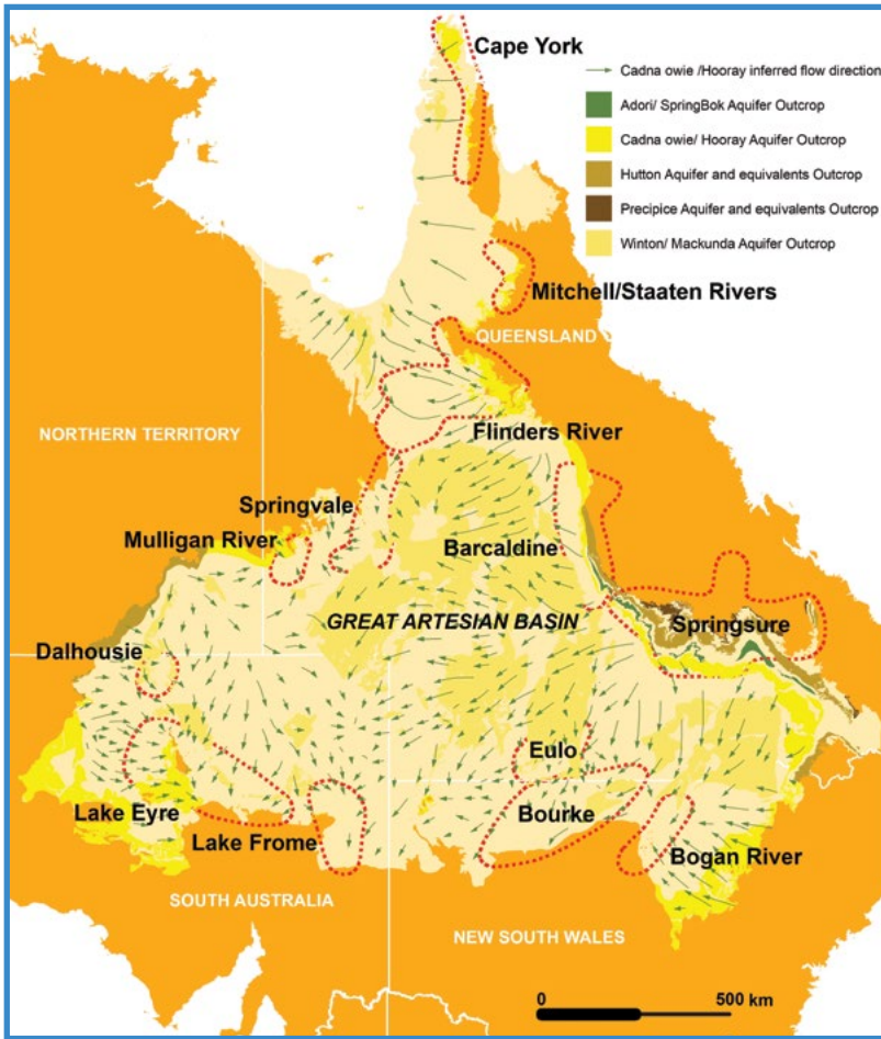
FIGURE 2 GAB SPRING SUPERGROUPS. Diagram showing the main GAB spring supergroups and how water flows from east to west across the Great Artesian Basin, from the Great Dividing Range towards Lake Eyre. (Figures constructed from data sourced from Ransley et al. (2015) 74 )
