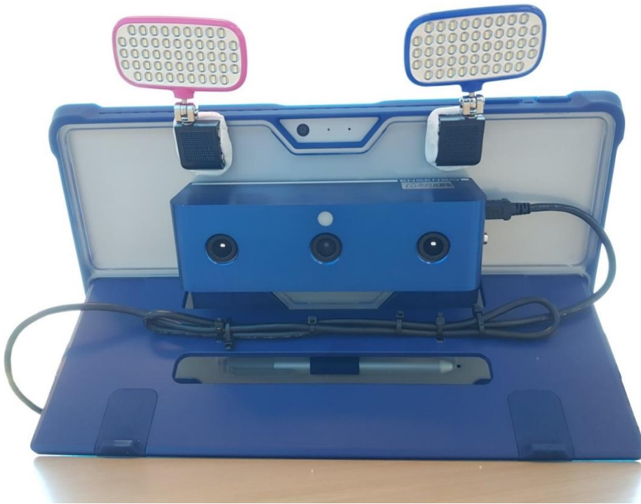
Figure 1.6. The WoundVue Camera: a 3D camera for diabetic foot ulcer wound measurement using the laser structured light technique (LBT Innovations Limited, Adelaide, Australia developed with the Australian Institute for Machine Learning, University of Adelaide)
