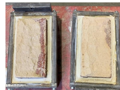
(ii) – Failed joint interface
