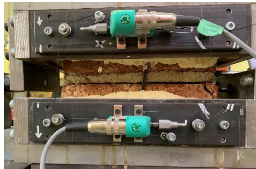
(i) – Elevation following failure
