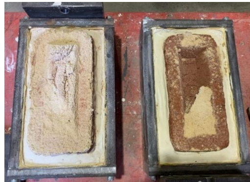
(ii) – Failed joint interface
