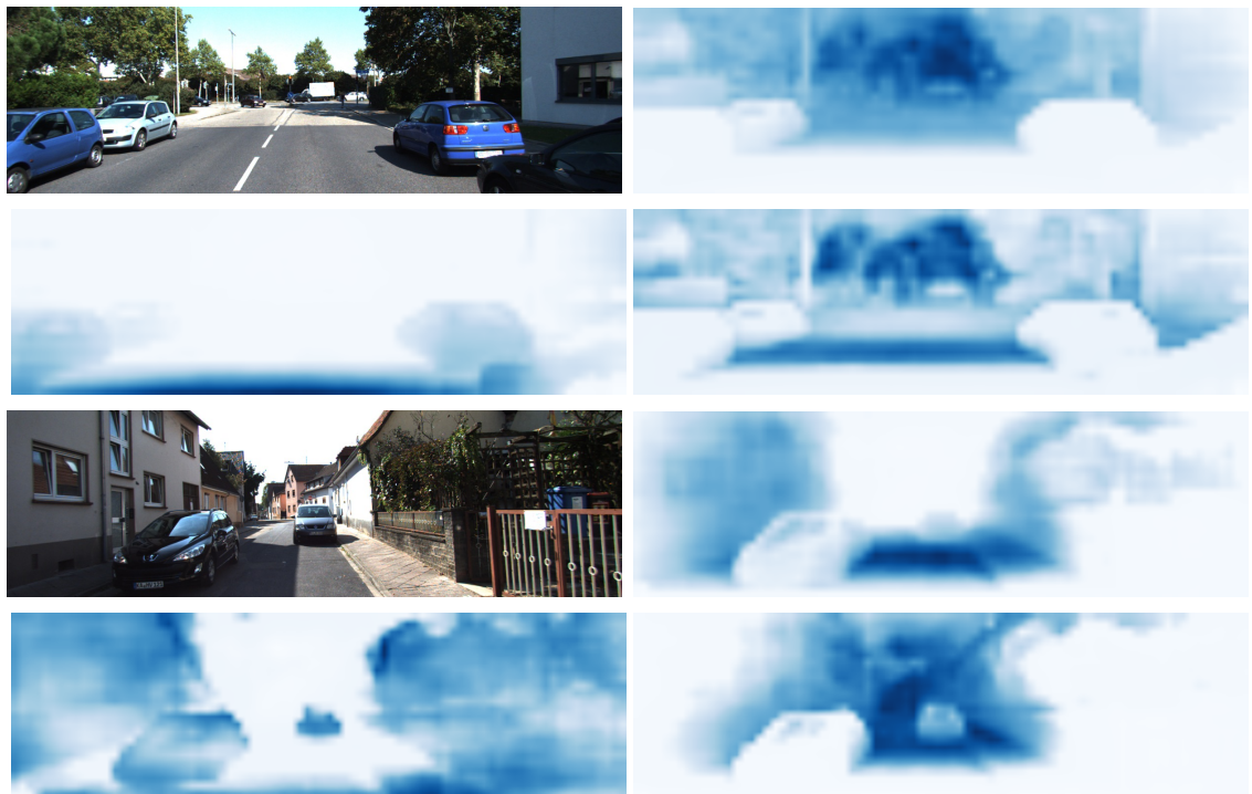
Figure 6.5: Attention maps from our network. Subset of the attention maps produced by our method. Blue indicates region of attention.
