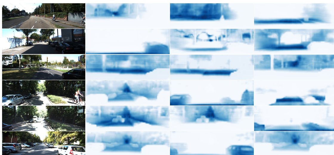
Figure 6.9: Additional attention maps selected at random from the output of context module (Blue indicates areas of high attention).
