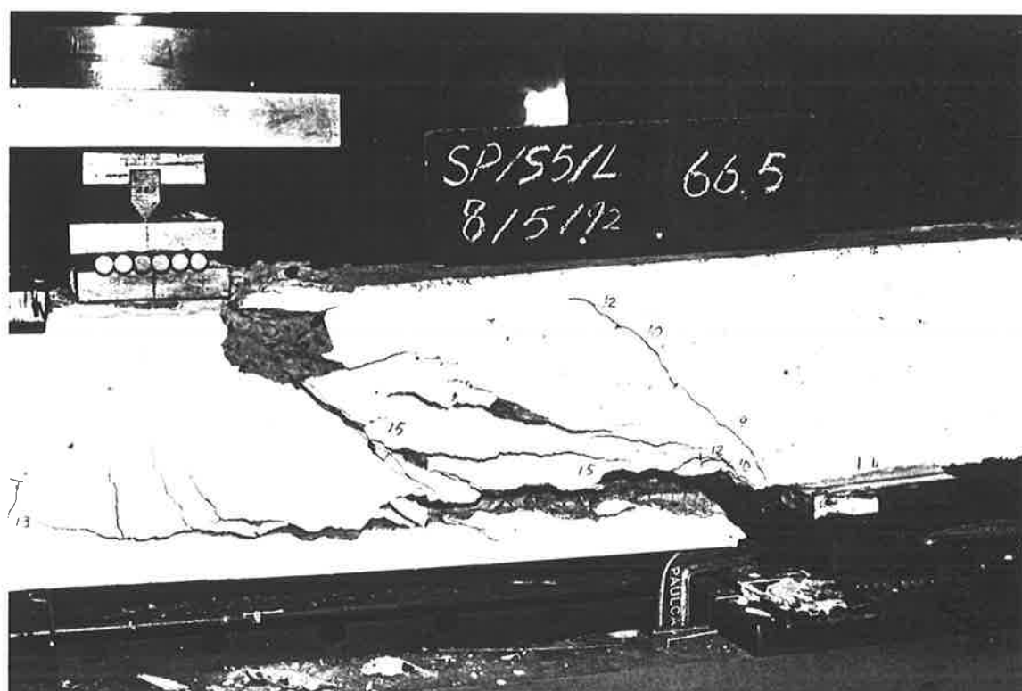
P3-70 The beam failed in shear
