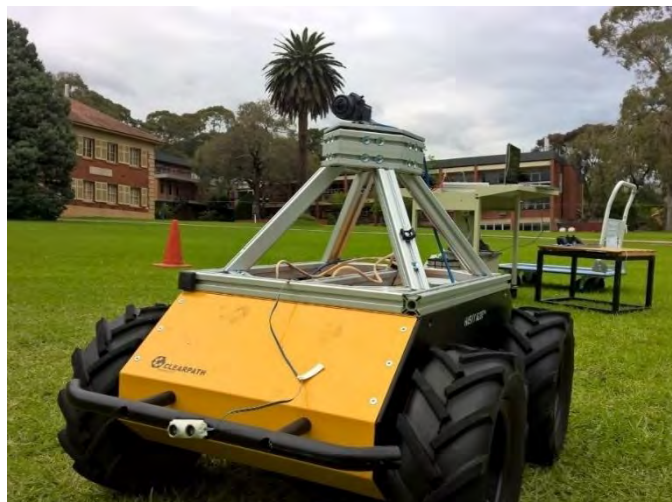
Figure 1.18. The insect-inspired target tracking model is implemented on a ground-based robot to autonomously track targets within natural environments.
