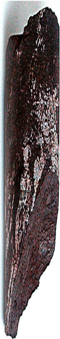
Figure 7: Depth/Thermal Conductivity Profile of Sample SDDD01-22 alongside the photograph of the dry sample. Note the smooth transitions between measurements but the large range of thermal conductivities exhibited by the sample ( 1.4 - 4.3 \text{ W/mK}^{-1} ), which is important to note considering the small size of the sample ( <15 \text{ cm} ). Note also the evidence of fluid pathways within the sample, indicated by the white markings on the core.
